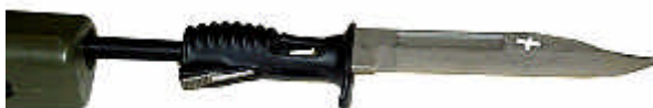
Fig.23. The L3A1 Bayonet Fixed. The bayonet also has a multi-tool facility as wire cutter and saw. (SAS 2180)
