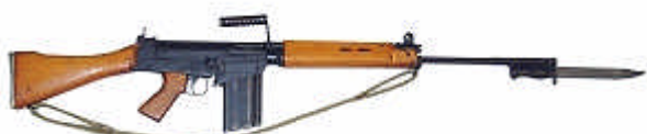
Fig.17. The Fabrique Nationale Fusil Automatique Légère bought by Britain in May 1954 and called the Self-Loading Rifle or 'SLR'. The bayonet is the L1A3. (SAS 2551)
