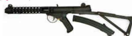
Fig.15. The 'Machine Carbine, L2A3' or 'Sterling Mk.4' derived from the Patchett 9mm calibre design of 1944. (SAS 952)
