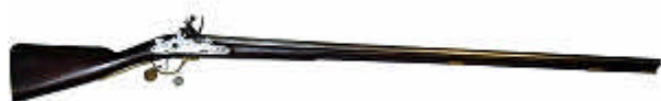
Fig.1 A 'dog lock' musket from the reign of Queen Anne (1702-1714). This had a plug bayonet. (SAS 2387)
