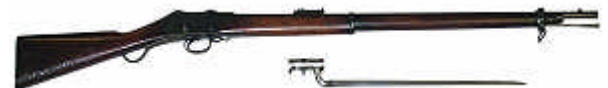
Fig.9. The 1 st Pattern Martini-Henry Rifle used with a bushed Pattern 1853 socket bayonet from 1872. (SAS 358)
