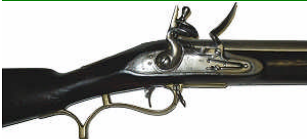
Fig.6. The flintlock of the Baker Rifle. (SAS 21)
