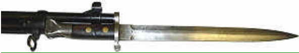
Fig.11. The Pattern 1888 bayonet mainly used on the Lee-Metford and Lee-Enfield Rifles of 1892 and 1895. (SAS 0371)
