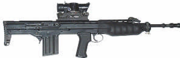
Fig.19. An experimental version of the SA 80 (XL64E5) which used a bowie bladed socket bayonet during trials in 1976-1978. (SAS 2041)
