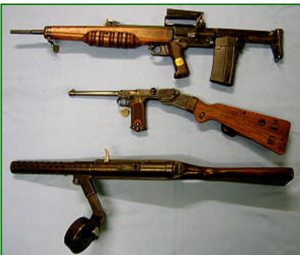
TOP 7mm Enfield Model 2 c1950 MIDDLE 7.65mm Borchardt c1893 BOTTOM 9mm Bergman MP 18 c1918
