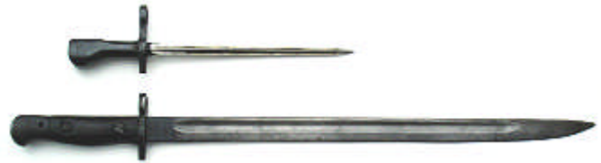
Fig.4. The experimental bayonet for a shortened P.1914 rifle circa.1924 (SAS 556) compared with the Pattern 1907 of Rifle, Short, Magazine, Lee-Enfield . The latter originally had a forward curved quill on. (Courtesy John Humphries)
