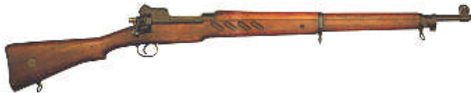
Fig.1. Rifle, Magazine, Enfield, .276-inch, Pattern 1913. (SAS 968- Courtesy of the Trustees of the Weapons Collection, Warminster)
